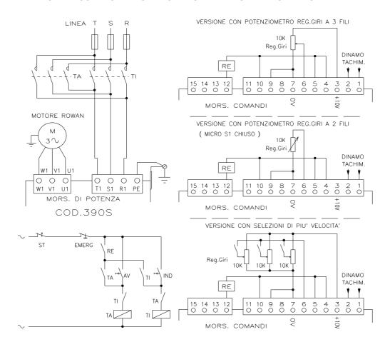
This type of operation foresees speed adjustment using an external potentiometer and selection of the rotational sense with the forward run (TA) and backward run (TI) electromagnetic switches.
