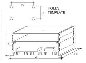
NB: The power unit installation must guarantee an air change.
