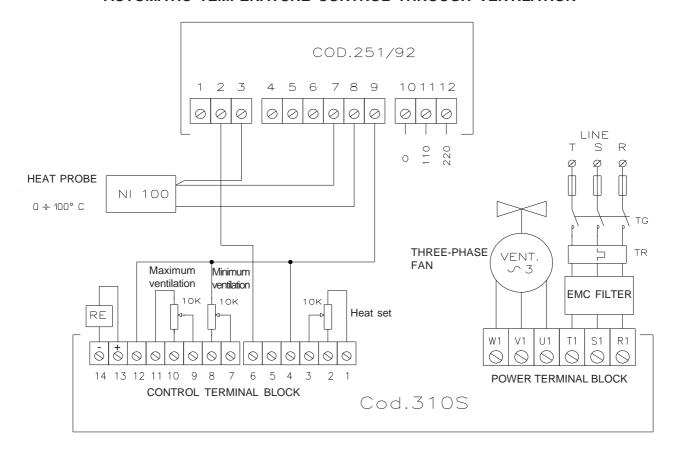
This layout is used for temperature control in zootechnical and industrial environments. CODE 310S, in **CLOSED-LOOP** configuration, is used as a heat probe for the control of parallel-connected fans having unit power of not more than 0.75kW (see section about Fans on page 8); board CODE 251/92 acts as a transducer for the NI100 probe and supplies an output (terminals 6-9) 0VDC at 0°C and +10VDC at 40°C.
