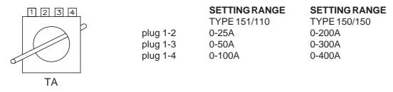
By performing several wire crossings you may modify the setting range thus adapting it to the various currents. For example: with 151/110 type TA plug 1-2 with 5 wire crossings, the setting range will be 0-5A (full scale divided by the number of wire crossings).
